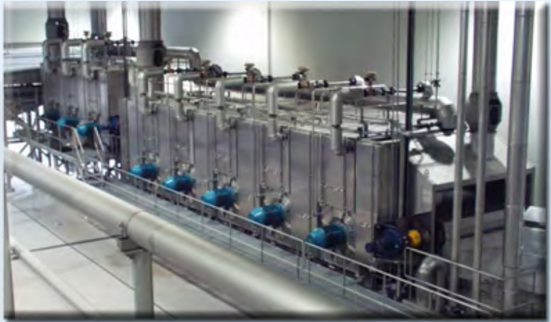
18T PER HOUR OUTPUT STAINLESS STEEL FRENCH FRY DRYER
