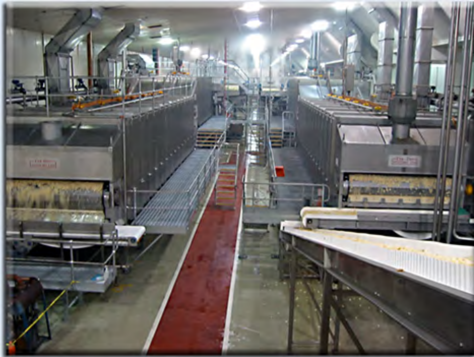
TWO 25T/HOUR OUTPUT ST. STEEL FRENCH FRY DRYERS
